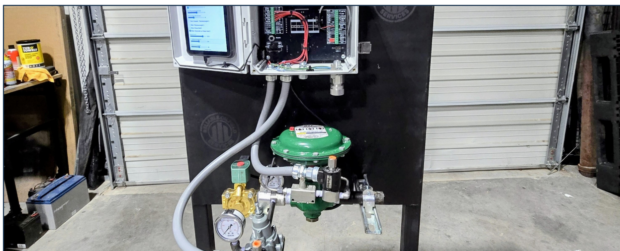
HEATER TREATER QUICK-CONNECT UNIT — BMS, TOUCHSCREEN, AND COMPLETE GAS TRAIN ON ONE STAND
